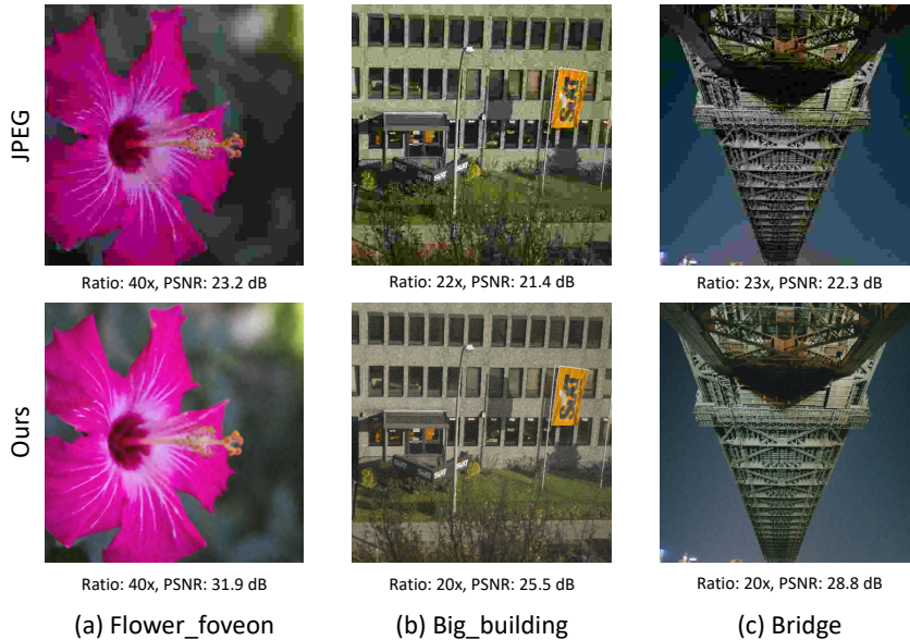
Figure 6: Qualitative comparison of JPEG versus our method in the low bit-rate regime. Unlike JPEG, the proposed approach does not lead to any block artefacts under severe compression. Compression ratios for our method are estimated, assuming weight reduction using RigL and int8 quantization—without any entropy coding. Quantization produces a fixed compression of 4\times , while sparsity is used as a toggle to achieve the target bit-rates. Zoom in to see details.
